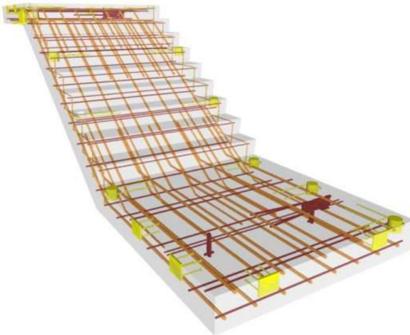
*LOD 400 Precast Structural Stairs (High Level of Detail) – Scaled fabrication modeling.*
